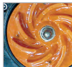
Tsurumi Impeller polished, not worn by abrasive material.
